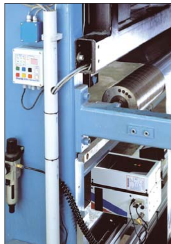
RTIS 2 unit firing onto vertical foil web.
