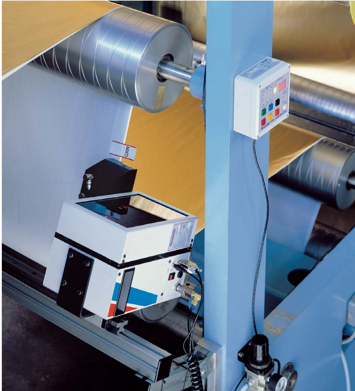
RTIS 2 mounted on a high speed foil application.
